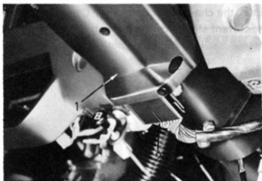
Fig. 3-16 Pulling Out 22-Terminal Connector
